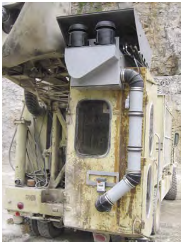
The installation of a unidirectional filtration system can greatly reduce a worker's exposure to harmful dust.
