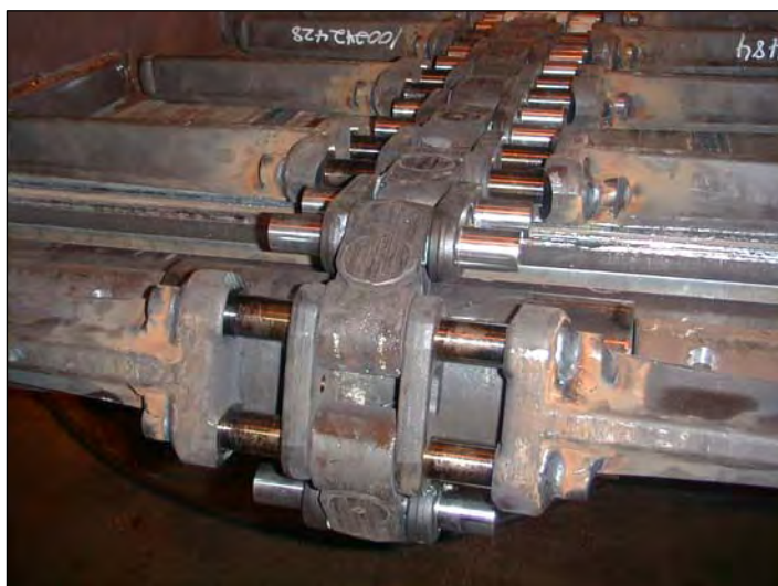
Figure 2.—Dual-sprocket driven chain.
