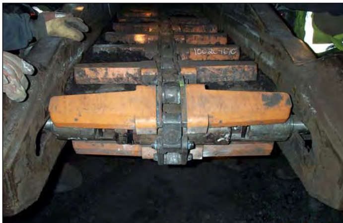
Figure 1.—Urethane-coated flight bar chain.
