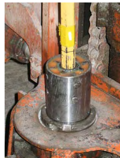
Figure 17 - Chuck isolator 2, 45 Shore A polyurethane filled
