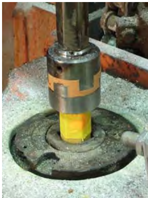
Figure 5 - Jaw-type coupling with 58 Shore D urethane spider
