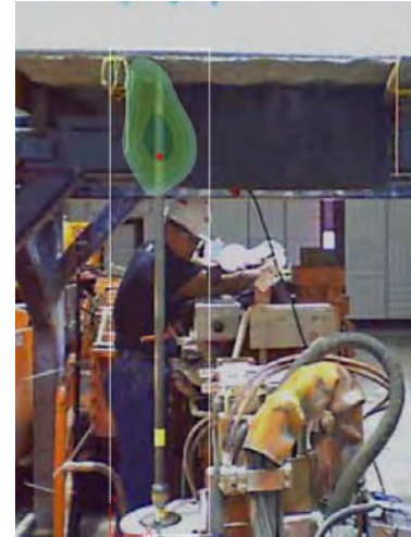
Figure 9 - Beamforming of drilling with the jaw-type coupling, 96 dBA @ the operators' position
