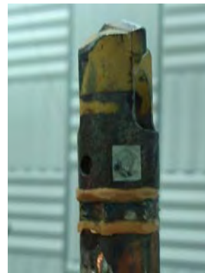
Figure 10 – Bit isolator with 60 Shore D urethane coating
