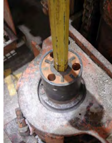
Figure 15 - Chuck isolator 1, 58 Shore D polyurethane filled
