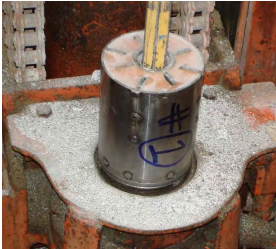
Figure 18 – Chuck isolator 3, 45 Shore A polyurethane filled, used for field testing and dose accumulation model
