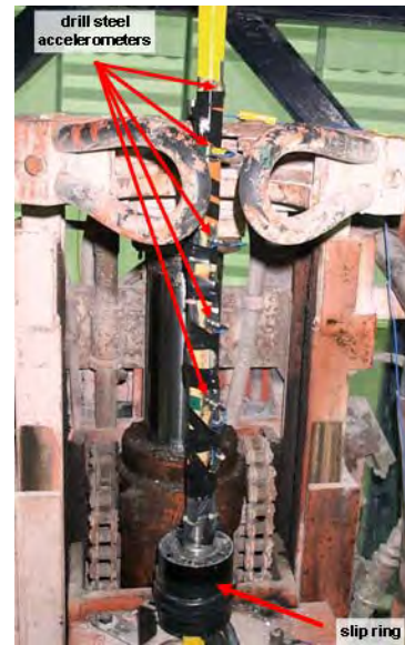
Figure 3 - Drill steel accelerometers and slip-ring assembly
