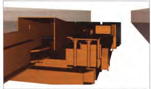
Figure 5: Operator's eye view, which allows the researchers to analyze the positions that the miner takes trying to see VALs while operating the machine.
