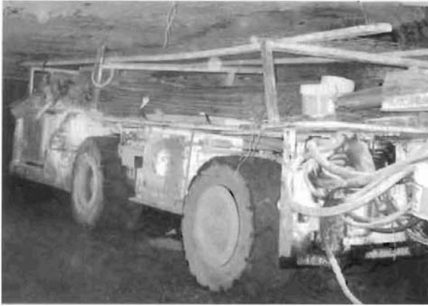
Figure 3: Roof bolter equipped with roof screen storage rack.
