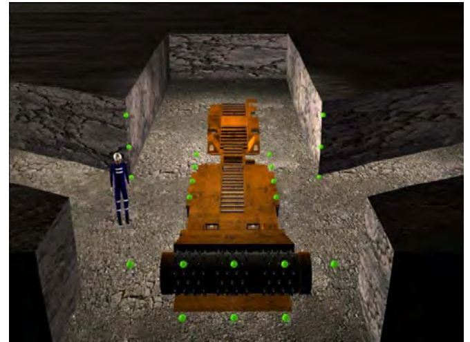
Figure 3 Simulated operator with visual cue matrix
