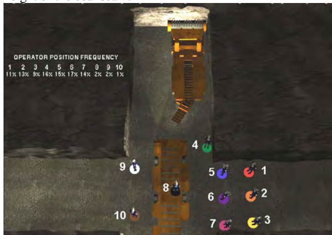
Figure 2. Available operator positions in cutting mobile haulage configuration.
