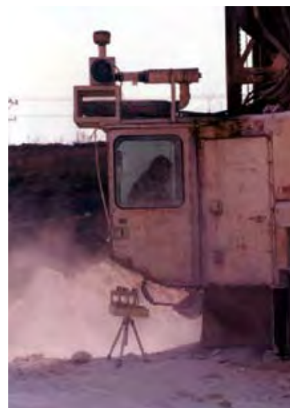
Figure 1. Cab filtration and pressurization systems prevent dust from penetrating cabs.
