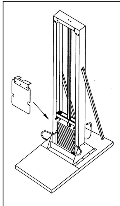
**Figure 4**—Incremental Weight Lift Machine. The barrier has been removed to expose the stack of weights. (Reprinted from **McDaniel, J.W., R.J. Shandis, and S.W. Madole: Weight Lifting Capabilities of Air Force Basic Trainees** (AFAMRL–TR–83–0001). Dayton, Ohio: Wright–Patterson AFB, Air Force Aerospace Medical Research Laboratory, 1983.)
