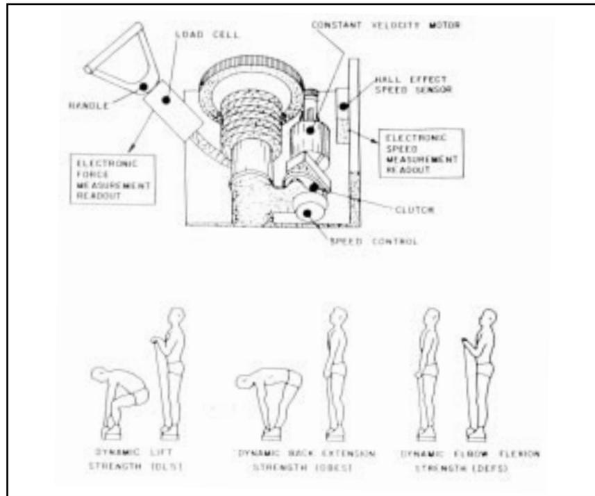
**Figure 8**—An isokinetic whole-body strength measurement system. This device allows the experimenter to assess various muscular strengths (such as those shown) at a constant velocity. (From **Kamon, E., and Pytel, J.L.:** Dynamic Strength Test as a Predictor for Maximal and Acceptable Lifting. *Ergonomics* 24(9):663–672 (1981). Reprinted with permission of Taylor and Francis Ltd.)
