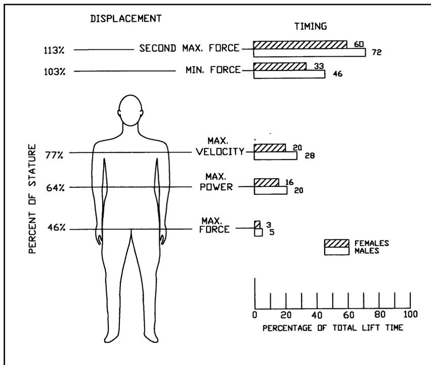
**Figure 5**—Displacement and timing parameters for a 1.83 m maximal isoinertial lift. Figure illustrates anatomical landmarks for the location of key events, found to be consistent for both genders. (From **Stevenson, J.M., et al.:** Dynamic Analysis of Isoinertial Lifting Technique, *Ergonomics* 33(2):161–172 (1990). Reprinted with permission of Taylor and Francis Ltd.)
