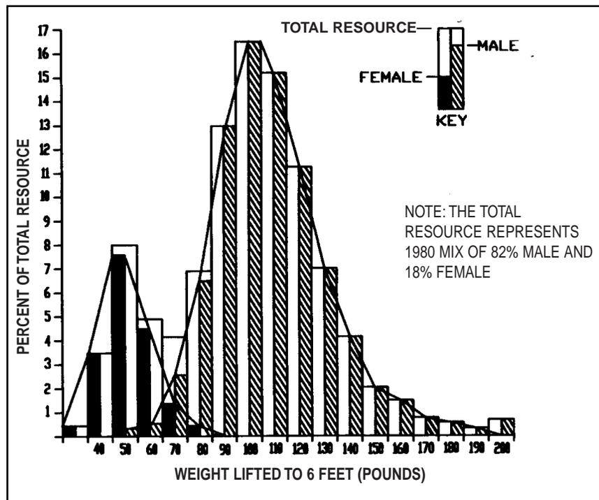
**Figure 6**—Distribution of weight lifted in a 1.83 m maximal isoinertial lift for male and female United States Air Force recruits. (Reprinted from **McDaniel, J.W., R.J. Shandis, and S.W. Madole: Weight Lifting Capabilities of Air Force Basic Trainees** (AFAMRL-TR-83-0001). Dayton, Ohio: Wright-Patterson AFBDH, Air Force Aerospace Medical Research Laboratory, 1983.)
