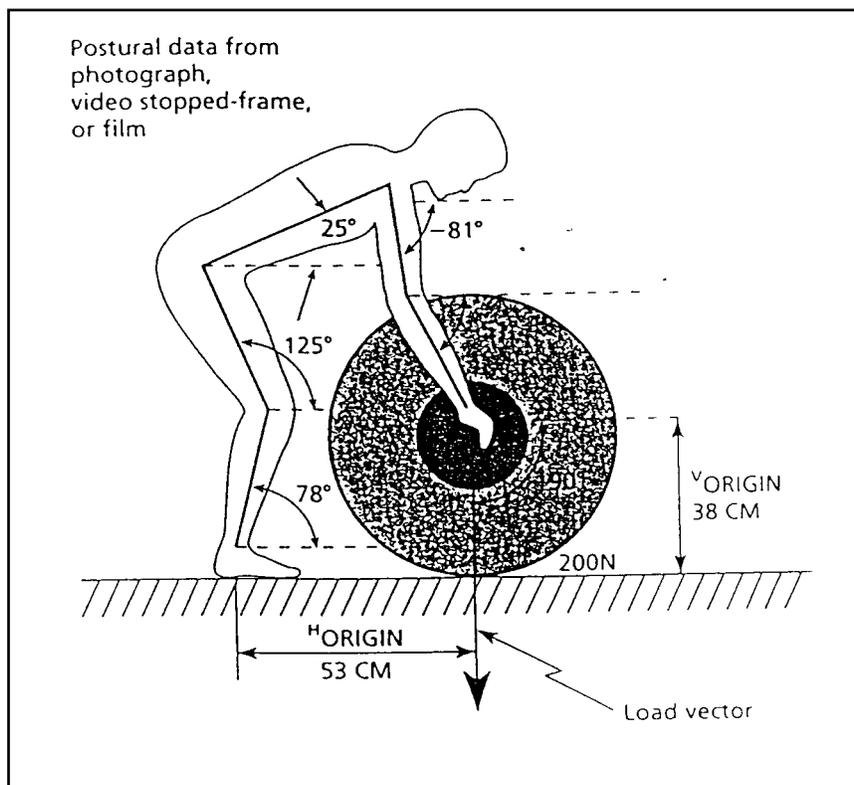
**Figure 2**—Postural data required for analysis of joint moment strengths using the isometric technique. (From *Occupational Biomechanics*, Chaffin, D.B., and G.B.J. Andersson, ©1991 by John Wiley & Sons, Inc. Reprinted by permission of John Wiley & Sons, Inc.)
