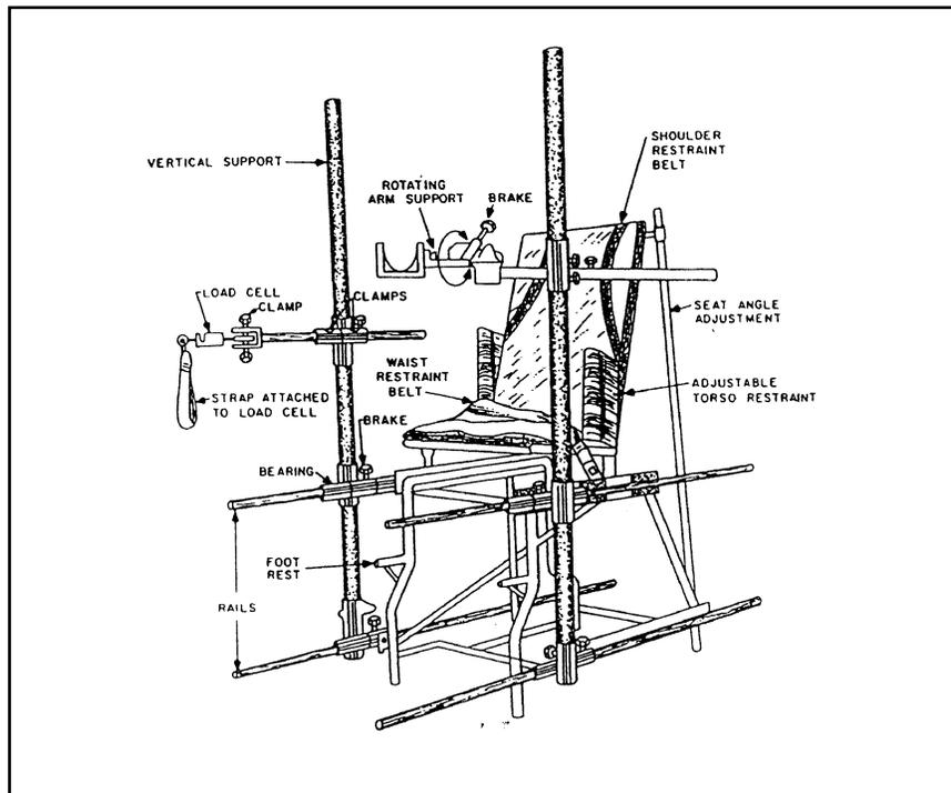
**Figure 3**—Example of a test fixture designed to restrain various body segments during isometric strength testing. (From *Occupational Biomechanics*, Chaffin, D.B, and G.B.J. Andersson, ©1991 by John Wiley & Sons, Inc. Reprinted by permission of John Wiley & Sons, Inc.)
