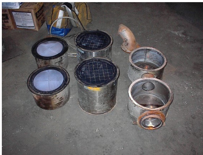
Figure 11 - ECS Octel DPF Components
