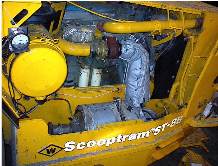
Figure 15 - DCL Bluesky Installation on VL247
