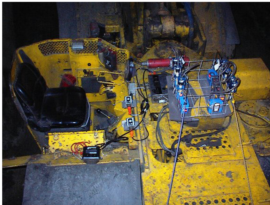
Figure 7 - RCD and NIOSH 5040 Operator DPM Sampling Trains
