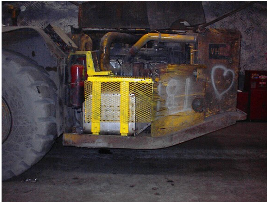
Figure 20 - Final Oberland Mangold DPF Installation
