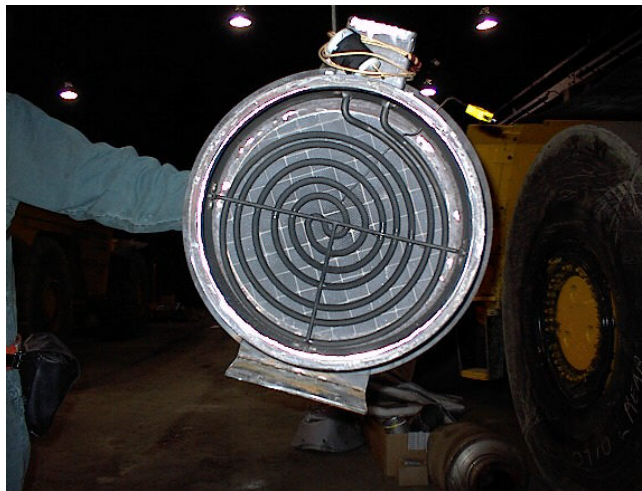
Figure 12 - DCL Bluesky DPF Silicon Carbide Monolith and Heater Element
