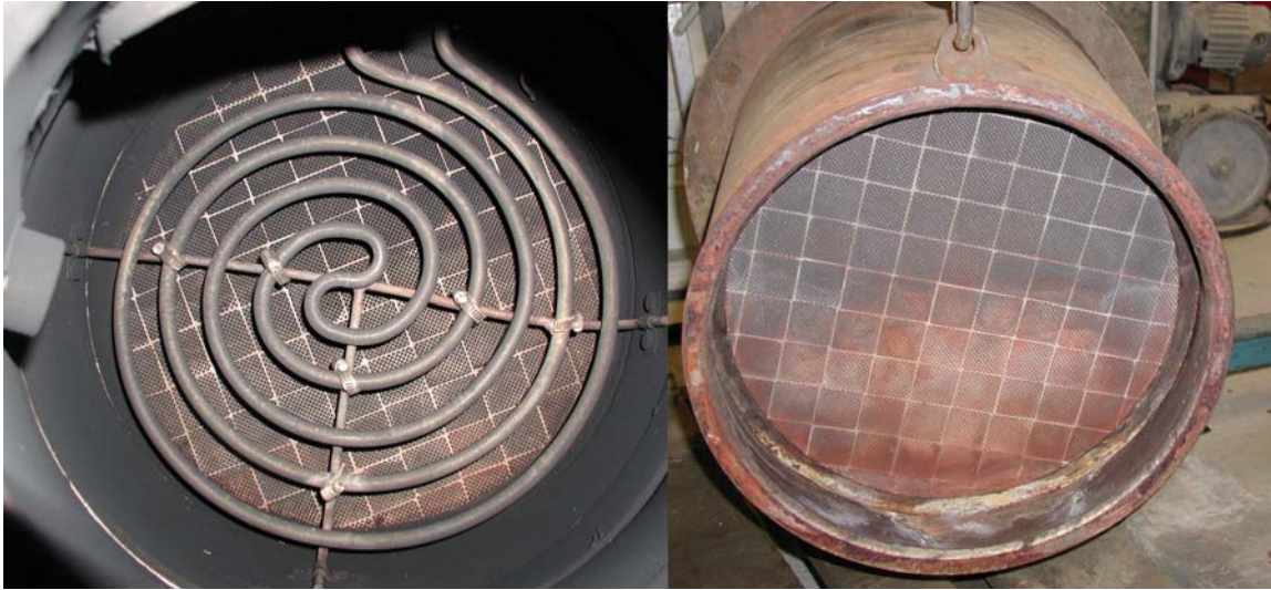
Figure 52 - Inlet and Outlet Faces of DCL Bluesky DPF
