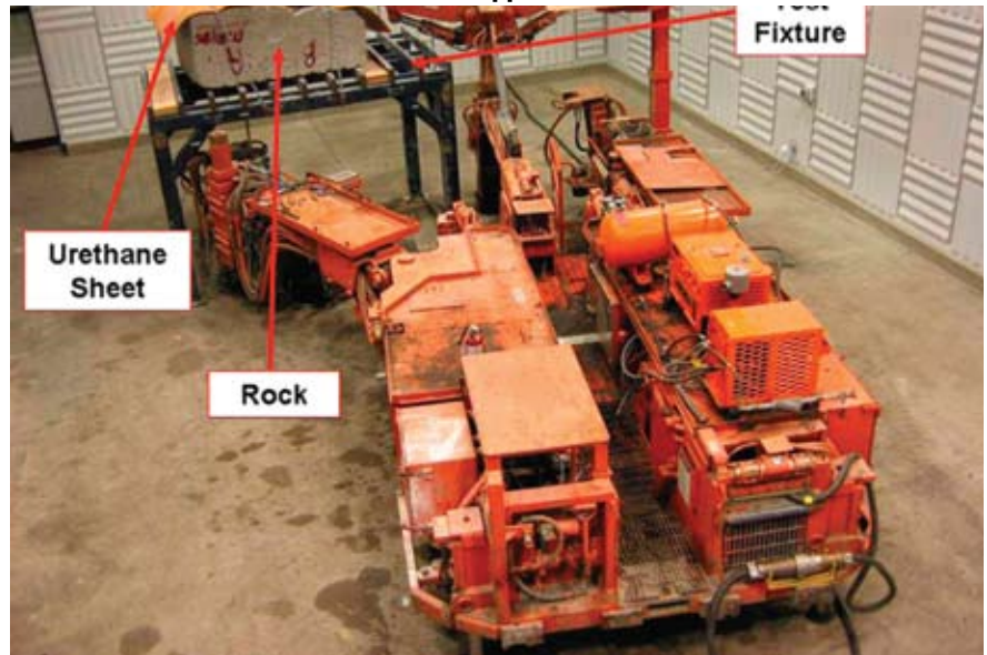
PRL's hemi-anechoic chamber and support stand for rock media.
