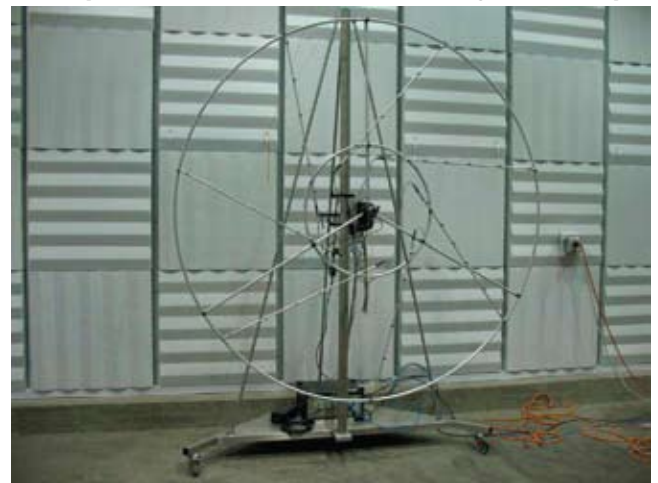
Forty-two channel acoustic beamforming wheel array.
