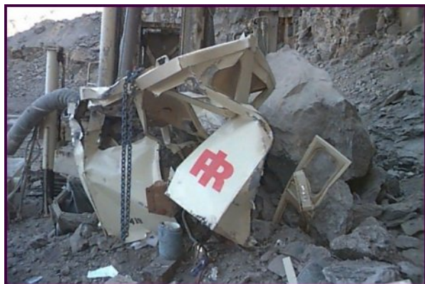
Figure 4: Cab crushed during slope failure (MSHA fatalgram, www.msha.gov ).
