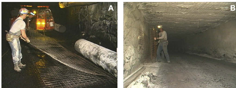
Fig. 1. Miners lifting wire mesh screen positioned on the mine floor (A) vs. stored upright against the mine wall, or “rib” (B).
