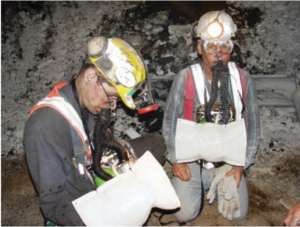
FIGURE 1. Miners wearing compressed oxygen SCSRs during a simulated escape
