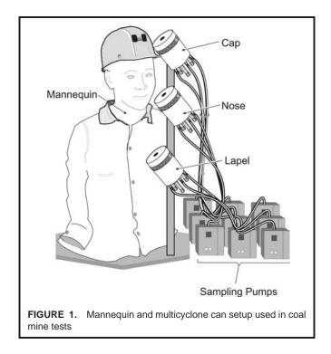
Three multi-cyclone sampling cans were mounted on the vertical shaft at the cap lamp, nose, and lapel of the mannequin. Each multi-cyclone sampler is made up of a metal can 10.8 cm in diameter and 12.7 cm high with a lid having a 1.9 cm diameter hole in its center. Each can contains cyclones and filter cassettes of three coal mine dust personal sampling units (CMDPSU) (Figure 2). A CMDPSU is made up of a 10-mm
