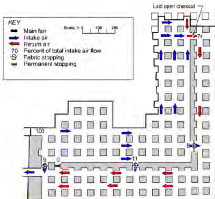
Figure 1. Blowing system using long pillars to direct ventilation air.
