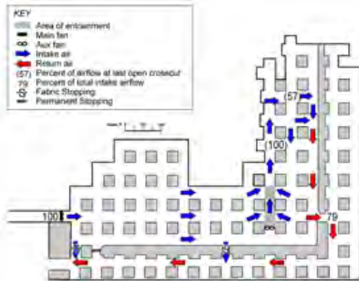
Figure 11. Face ventilation with properly positioned auxiliary fan.
