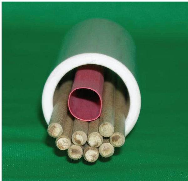
Figure 2.—Nine small ( 3/16 -inch) dowels and shrink tubing.
