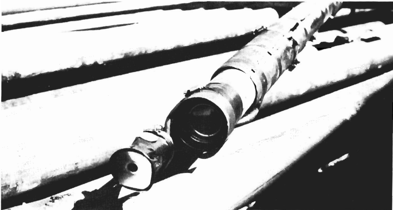
FIGURE 13. - Television camera. Light source in left foreground.
