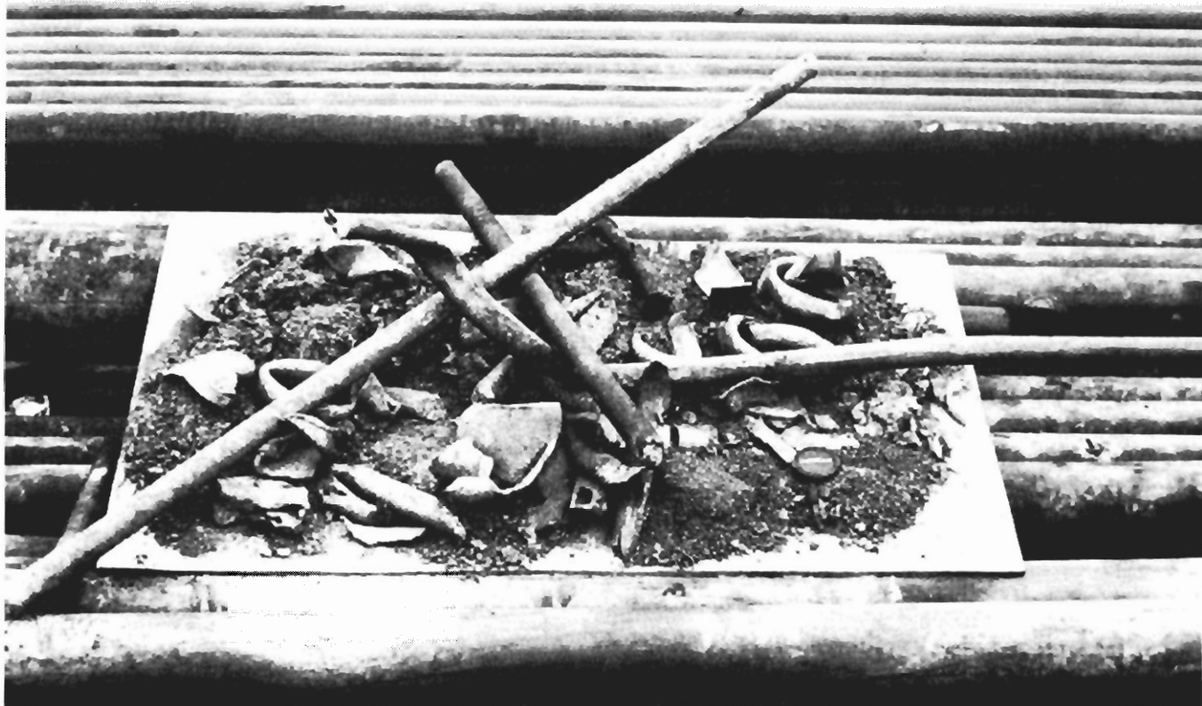
FIGURE 14. - Debris fished from EM-19. Long pieces were picked up by overshot and small pieces by magnet.
