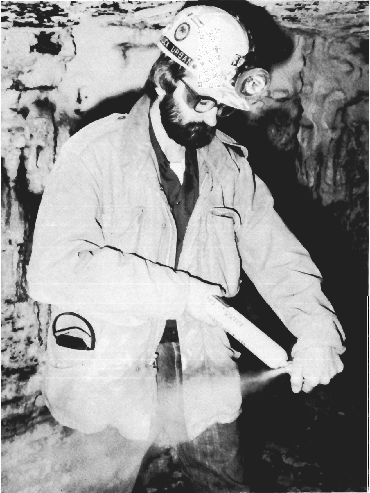
FIGURE 1. - Releasing SF 6 for ventilation analysis.
