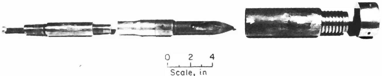
FIGURE A-5. - Alignment of snubber, mule shoe, orienting sub, and deflection shoe (left to right).
