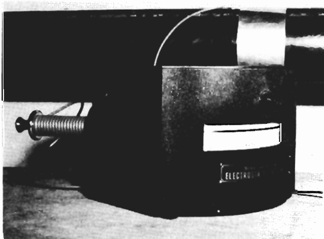
FIGURE 5. - Multirange electrostatic voltmeter.
