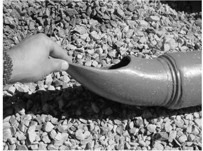
Figure 5. Elbow for bulk fill placement.
