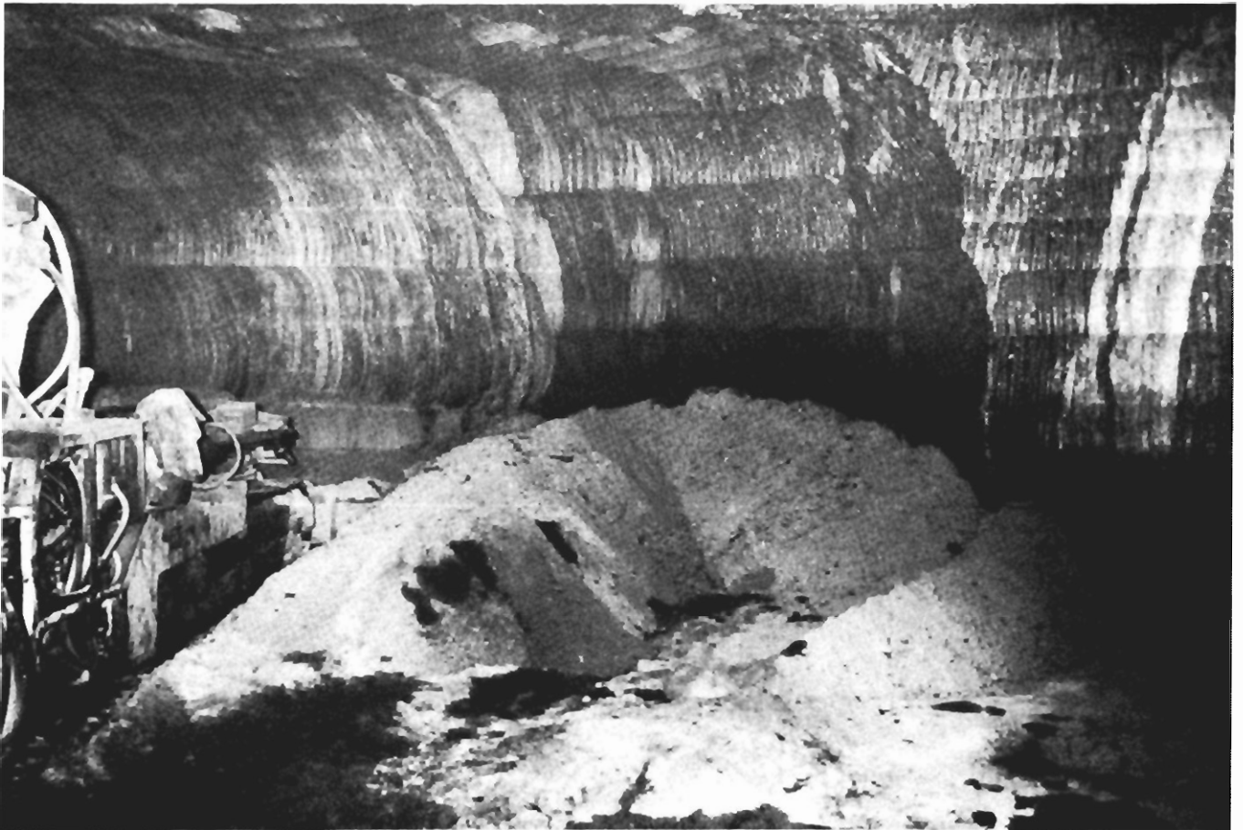
FIGURE 8. - Low-production-grade (wet-argillaceous) salt within anomalous zone of the decline.
