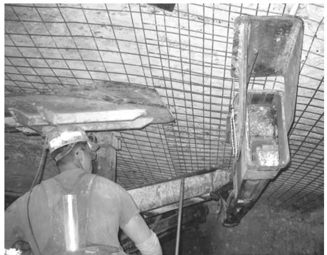
Figure 2. Screen providing protection during bolt installation.
