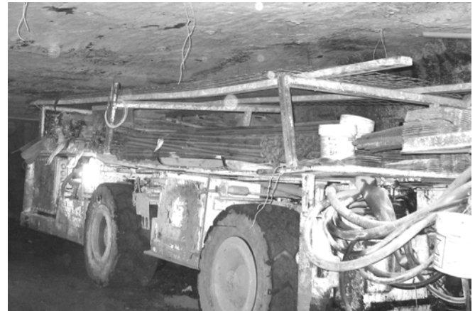
Figure 3. Rack used to hold and transport screen.
