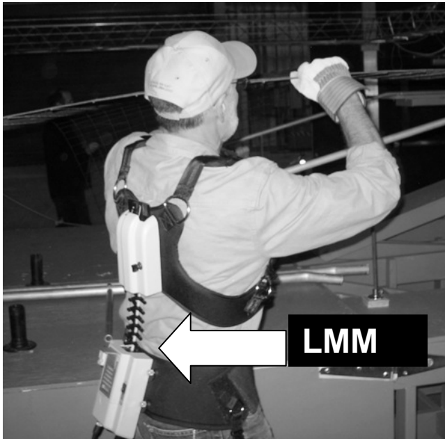
Figure 7. Test subject fitted with Lumbar Motion Monitor (LMM).
