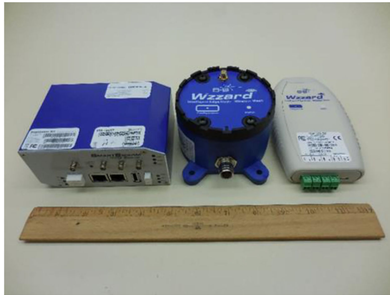
Fig. 3. A SmartSwarm cellular gateway (left), industrial-grade Wizzard node (middle), and commercial-grade Wizzard node (right)
