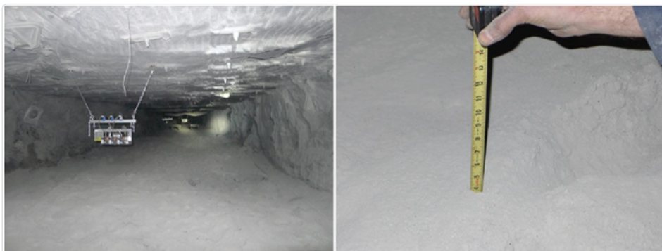
The photo on the left shows rock dust deposits on the roof, ribs, and mine floor at a field sampling location in a continuous miner air-ventilation return. On the right, a worker measures the deposits. Photos from NIOSH.
