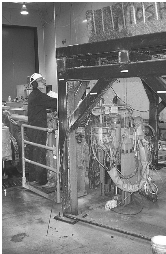
Figure 2 — Drilling support fixture loaded with granite.
