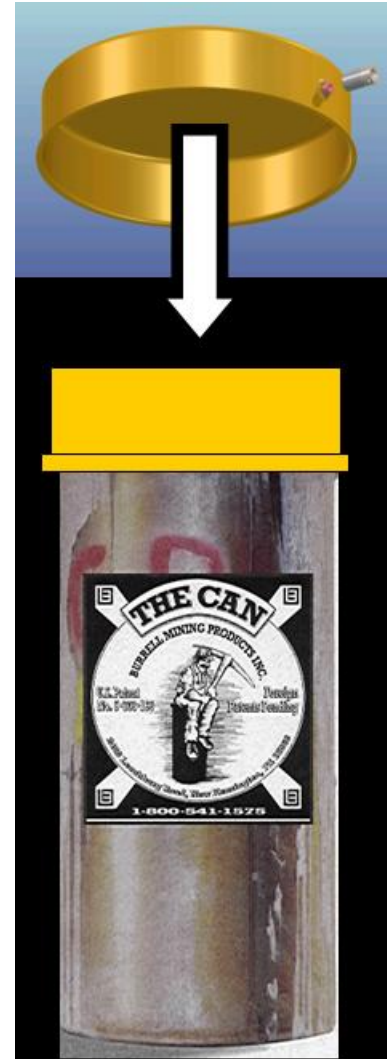
Figure 9. Diagram of a new PSU design for Can supports. This unit fits over the top of the Can like a cap and avoids issues caused by an oversized square PSU.
