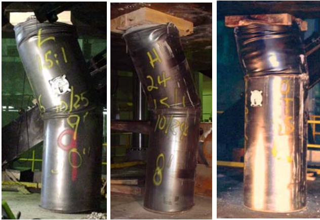
Figure 10. Buckling of Can caused by welding of sections together can create a hinge point during lateral displacement that may cause load shedding during yielding.
