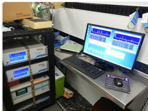
Three gas chromatographs, left, ready to report to work on-site. Photo from NIOSH.
