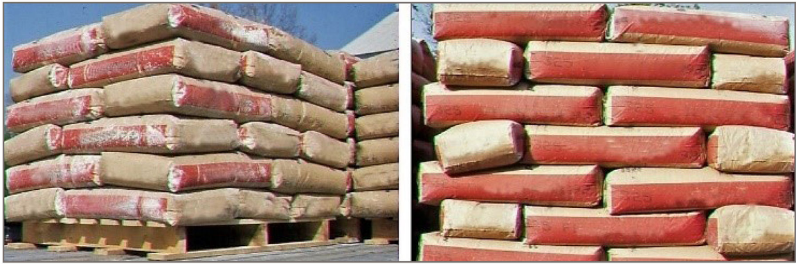
Figure 8. Pallet of bags without being cleaned by B&BCD system (left) and with being cleaned by the system (right).
