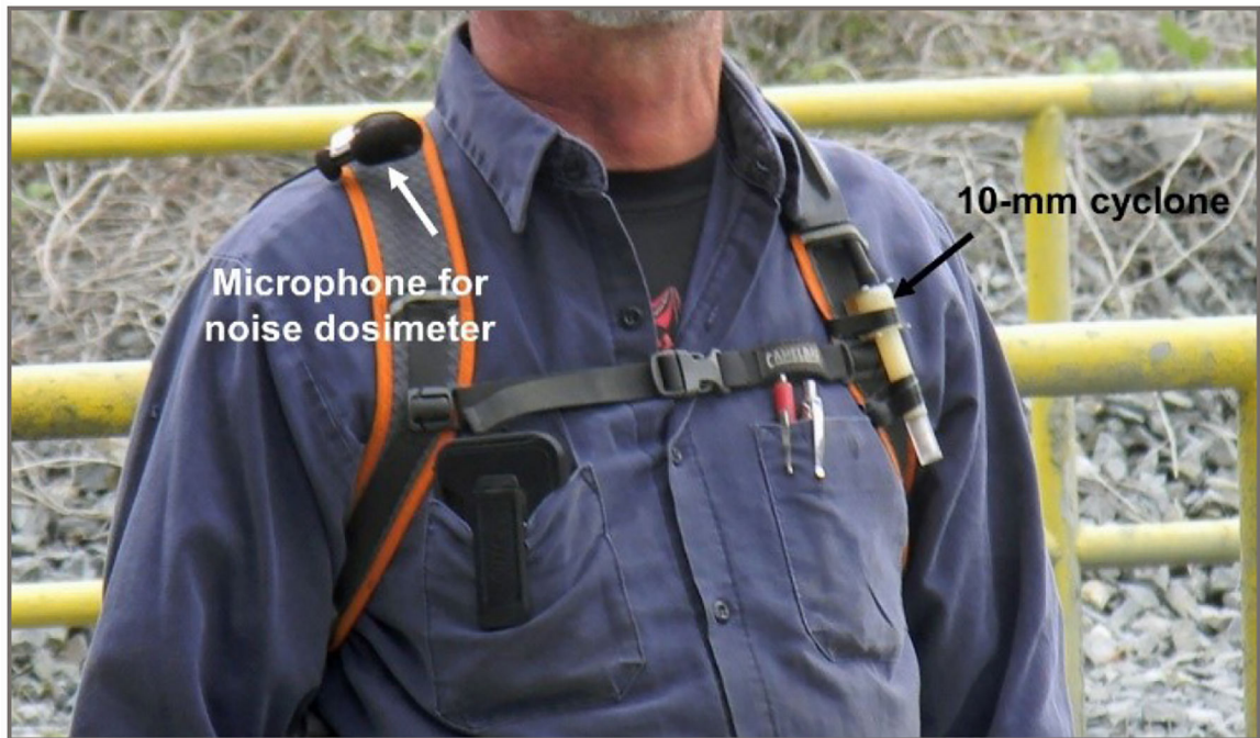
Figure 3. Simultaneous assessment of a miner's respirable dust and noise exposure using the Helmet-CAM system.
