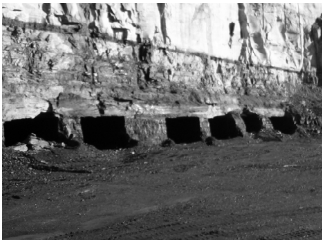
Figure 8. Typical highwall mining web and barrier pillars.
