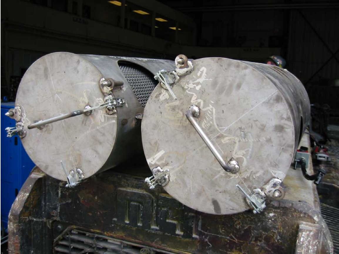
Figure 4 . Mac's Mining Repair/Donaldson P604516 filtration system on the LHD #92506
