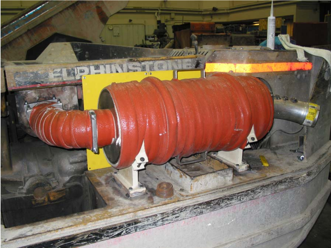
Figure 5. ECS Cattrap DPF system on the LHD #92526
