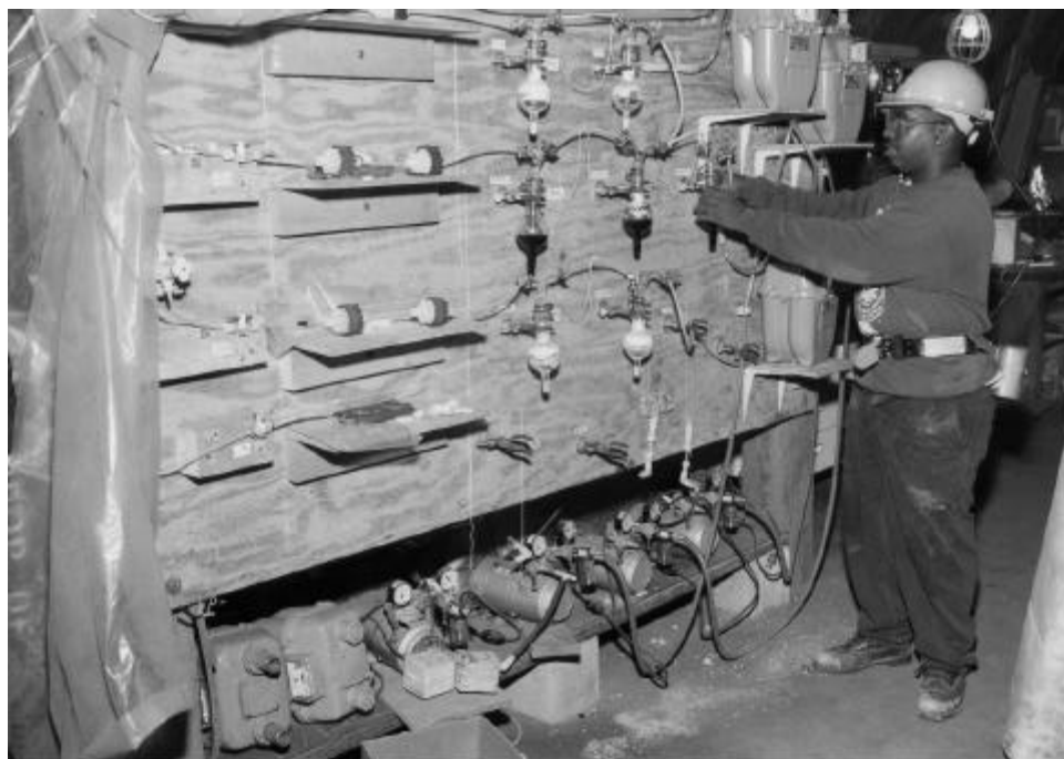
Figure 4. A series of bubblers were used to collect toxic gas components ( \text{NO}_x , \text{NO}_2 , and \text{NH}_3 ) that could not be collected in Vacutainers.
