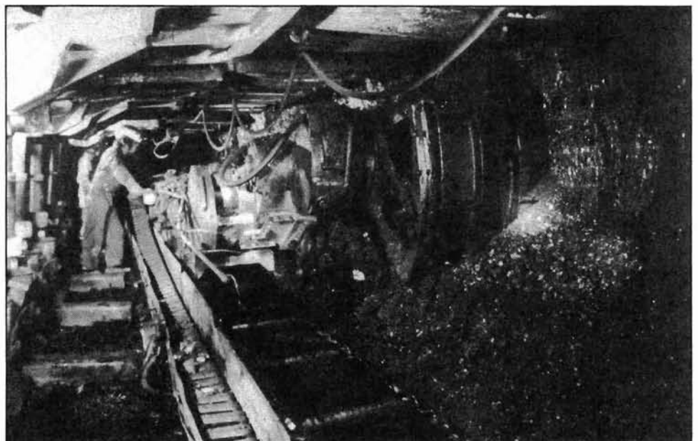
Figure 10.—Longwall shearer cutting coal.
