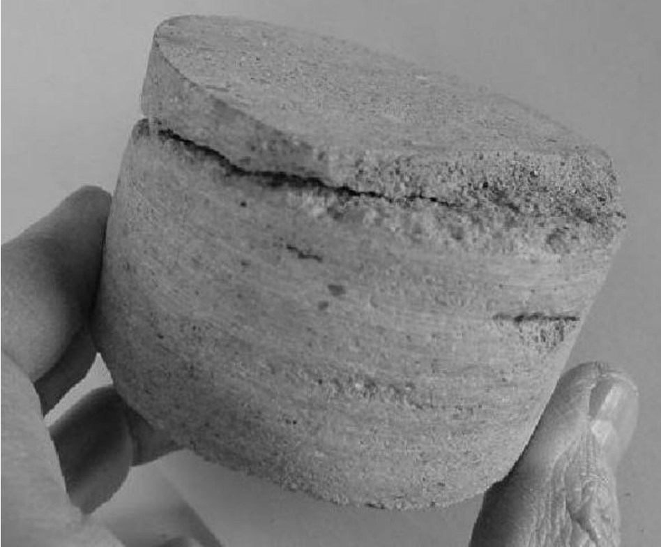
Figure 13 - Fine shotcrete coring with voids originating from poorly mixed material.
