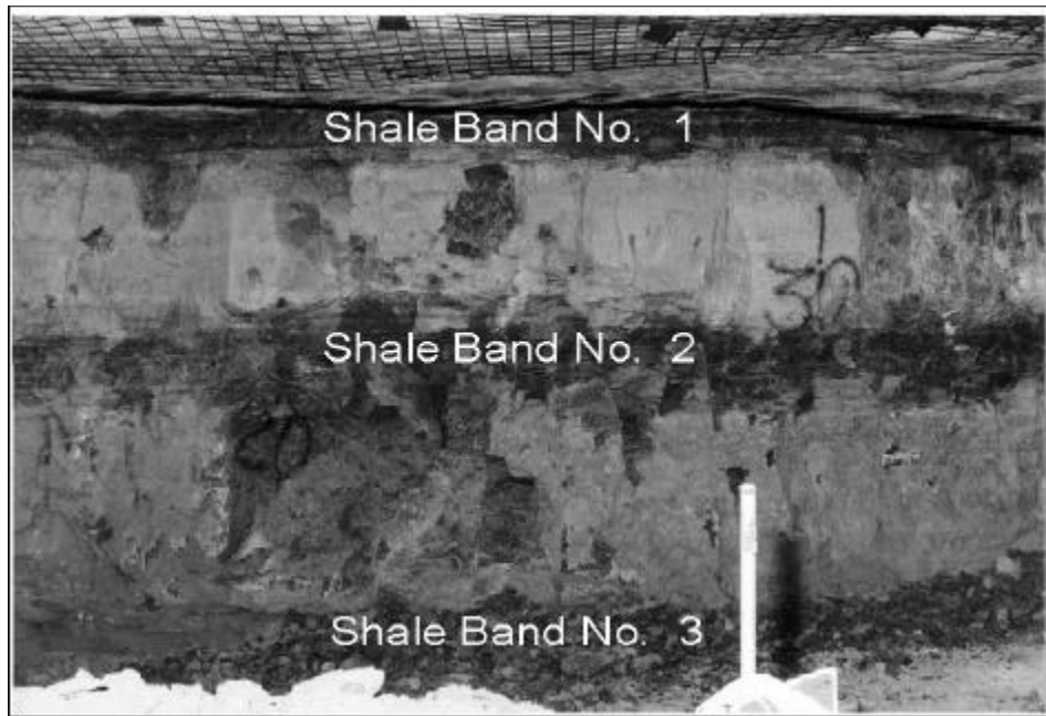
Figure 1 - Shale bands dividing limestone formation at LLEM.
