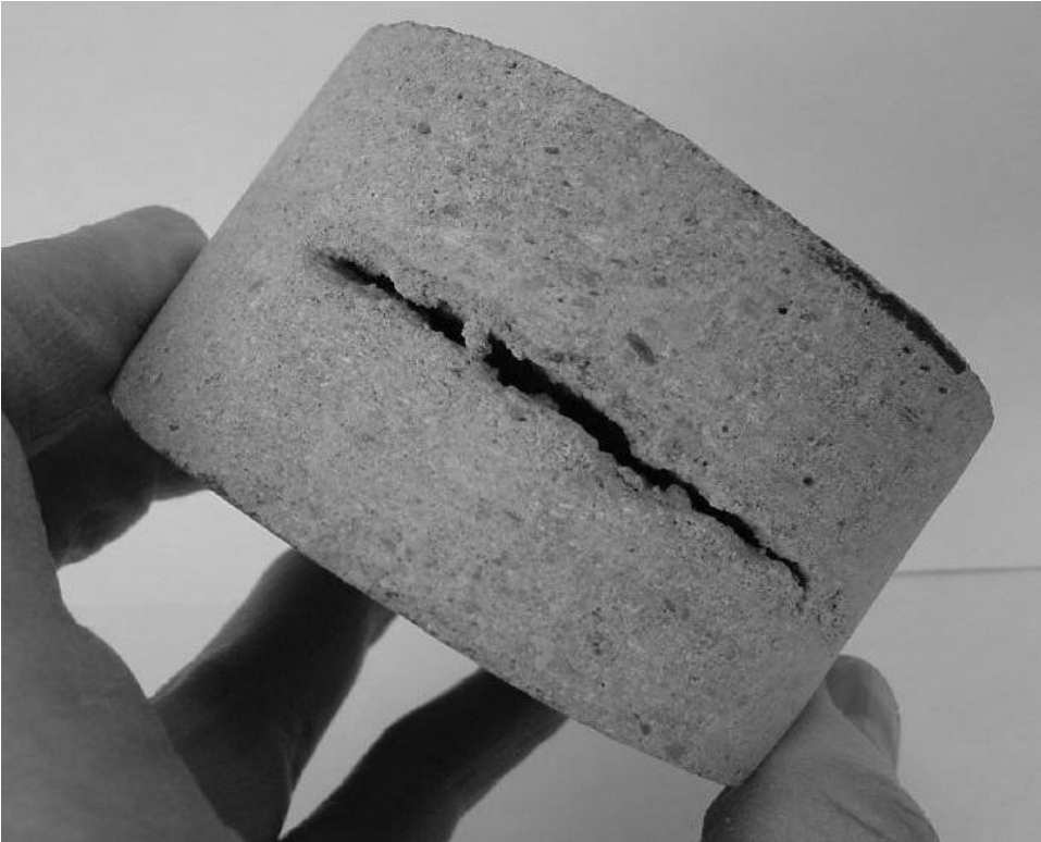
Figure 12 - Fine shotcrete coring with large void.
