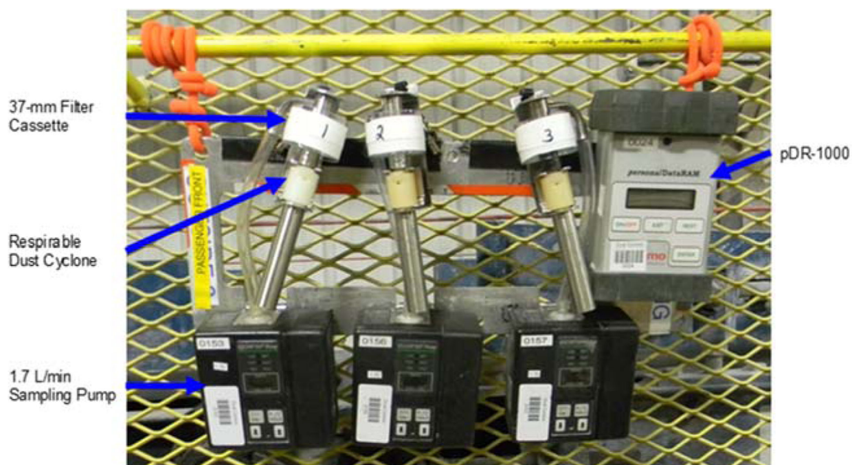
Fig. 6. Example of sampling racks with one pDR-1000 and three gravimetric sampling assemblies, including a sampling pump, a respirable dust cyclone, and a 37-mm filter cassette
