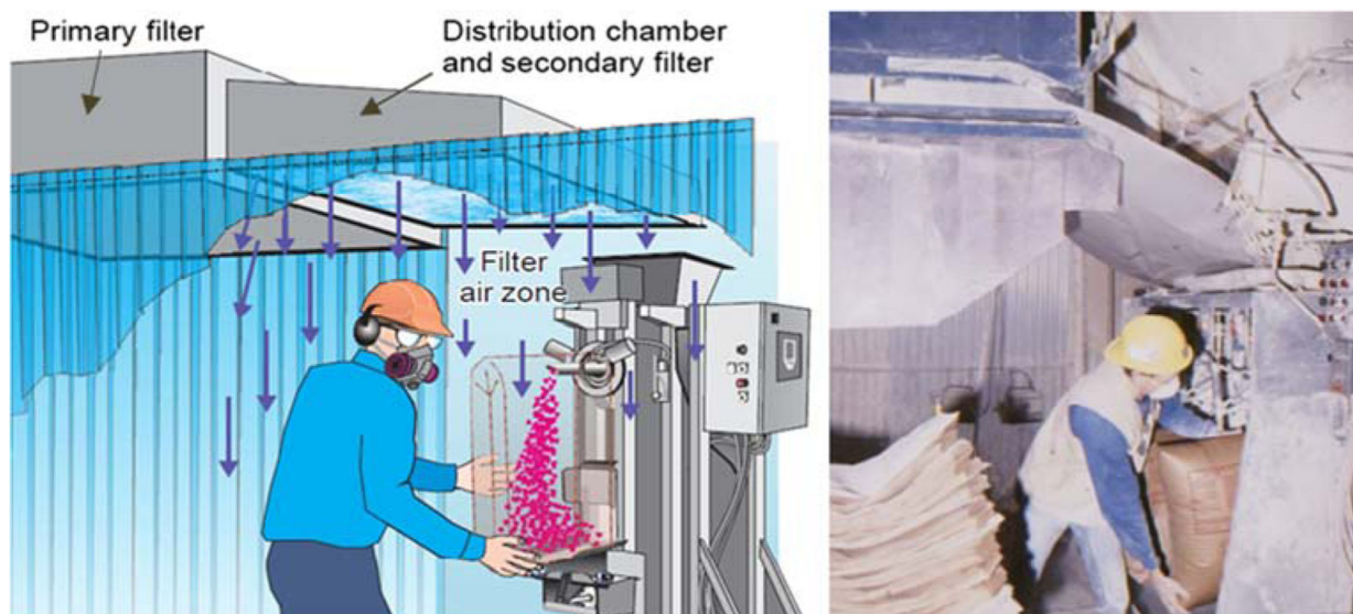
Fig. 3. Overhead air supply island system (OASIS). Left: diagram of system components. Right: OASIS positioned over bag operator
