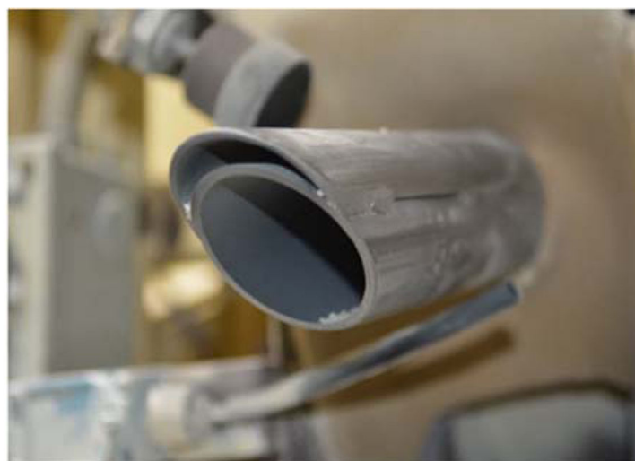
Fig. 2. Dual-nozzle bagging system. Left: Diagram of overall system components. Right: Close-up of a dual nozzle with an inner product fill nozzle and outer exhaust nozzle
