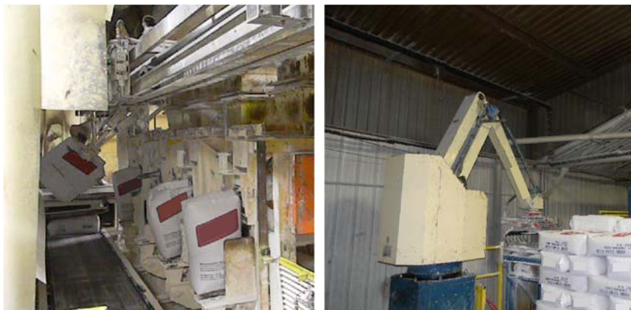
Fig. 11. Left: Automatic bag placer and filling station. Right: Robotic palletizing arm
