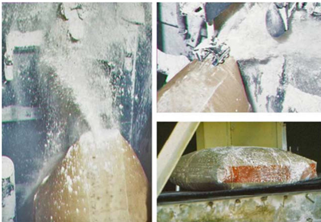
Fig. 1. Major sources of dust during valve bag filling. Left: Product “rooster tail.” Top right: Product blowback. Bottom right: contaminated bag
