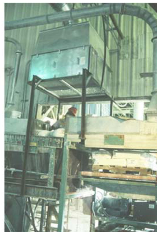
Fig. 5. Semi-automated bag palletizing system with OASIS and exhaust ventilation
