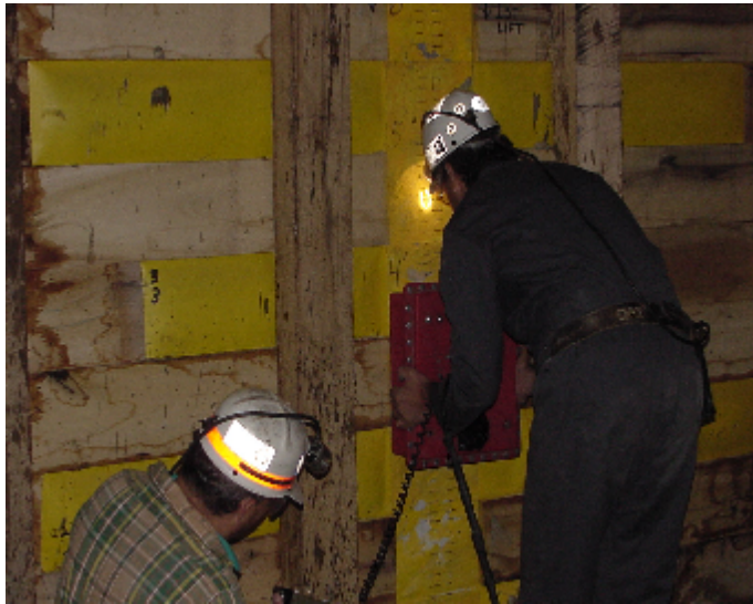
Figure 9. Researchers performing GPR scan of mine seal.
