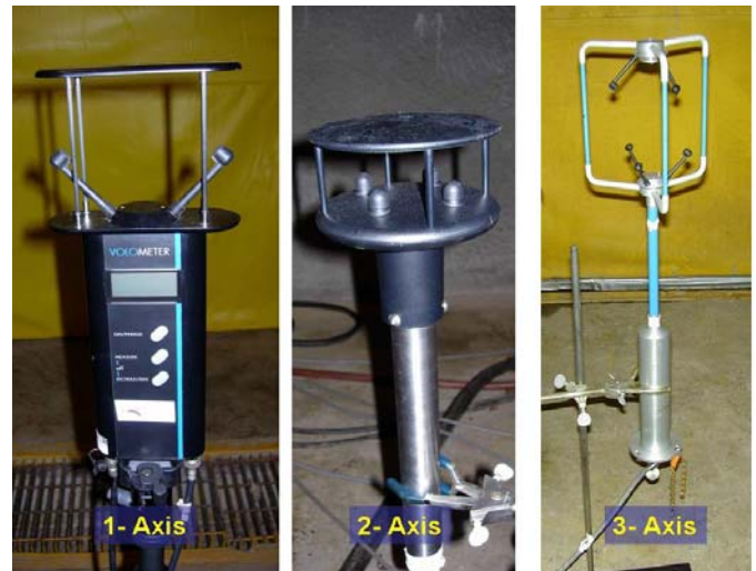
Figure 1. One-, two-, and three-axis ultrasonic anemometers.
