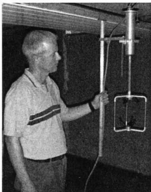
Figure 3 — Three-axis ultrasonic anemometer.
