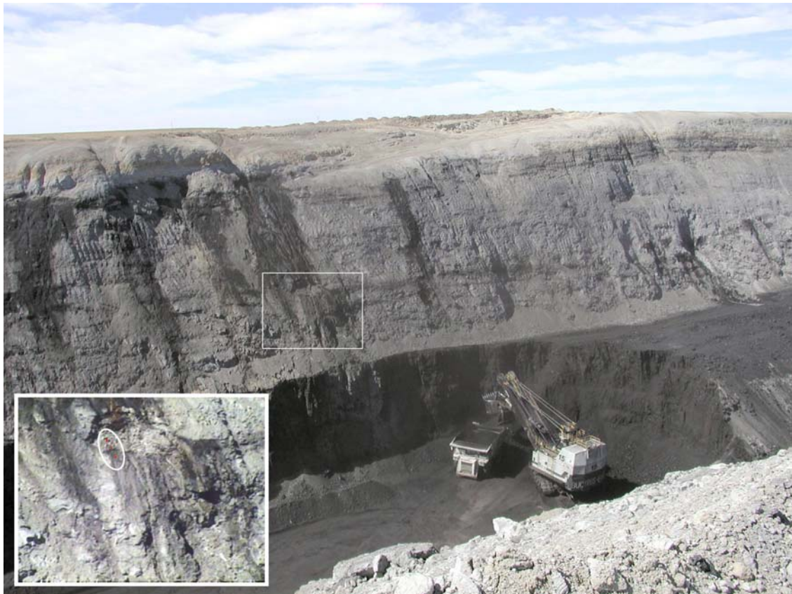
Figure 8.—Highwall at Black Thunder Mine. Box shows area of broken rock and water seepage monitored by video system. Inset shows video frame captured during detection of rockfall; area in oval shows where change was detected
