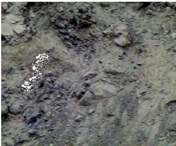
Figure 7.—Video frame captured during detection of rockfall in area of box shown in figure 6. Bright areas show where change was detected.
