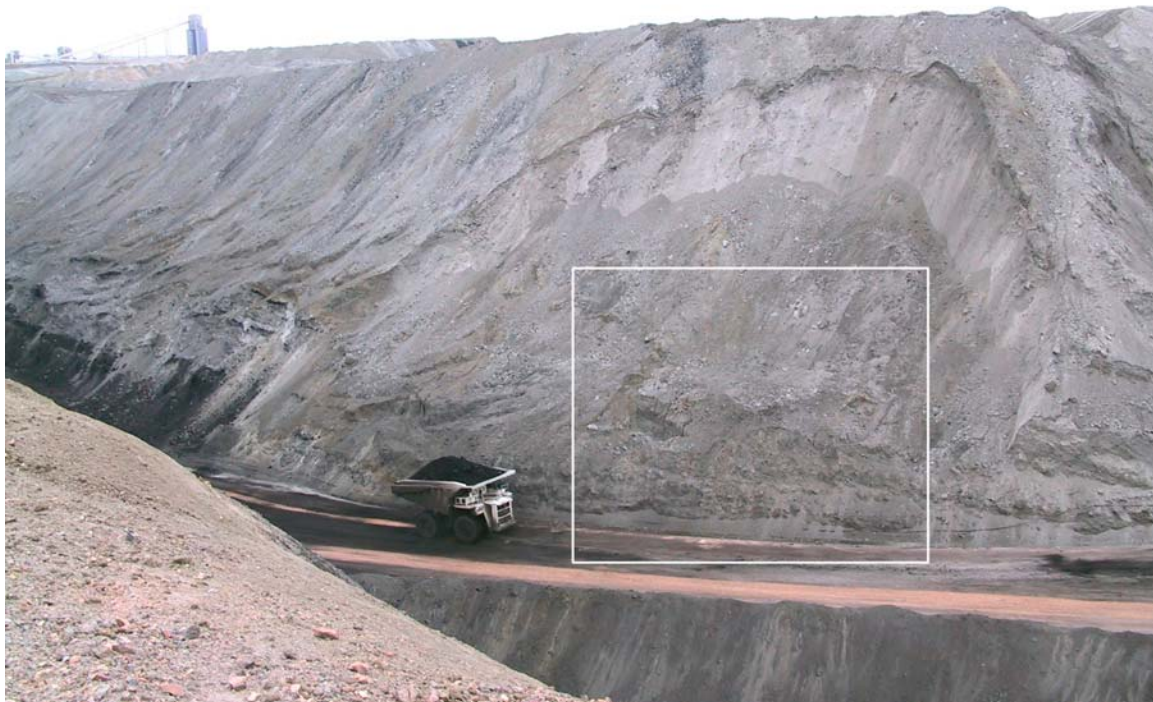
Figure 9.—Slump area in spoils at Black Thunder Mine. Box shows area covered by video monitor.
