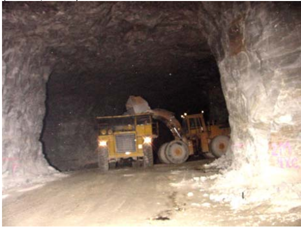
Figure 1. Typical large-opening mine entry [12.2 m x 8.2 m (40ft x 27ft)]
