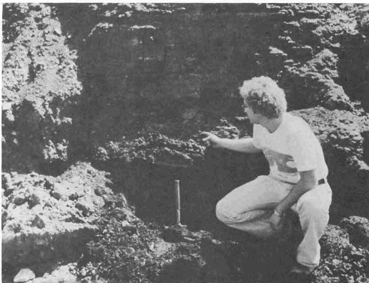
FIGURE 6. - Clay parting in the Lower Kittanning coalbed.
