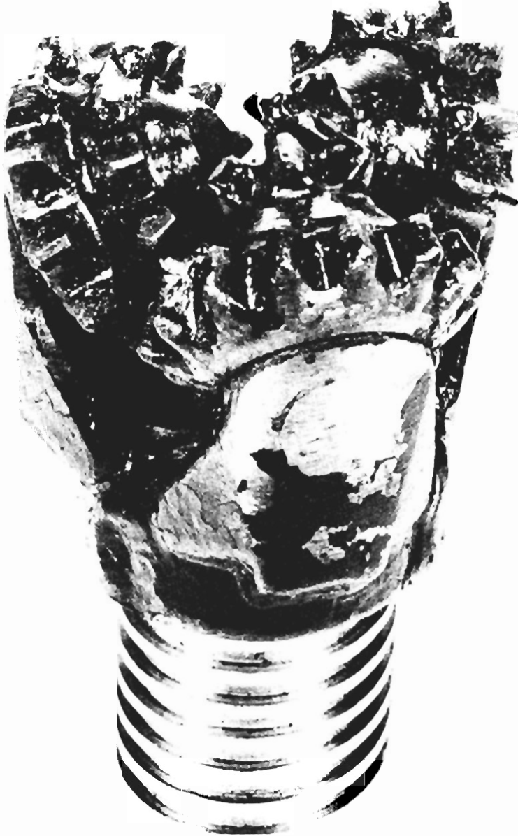
FIGURE 21. - Three-cone roller bit.
