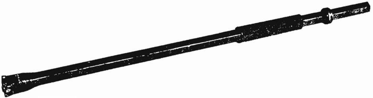
FIGURE B-22. - An unabated rod with a shoulder.
