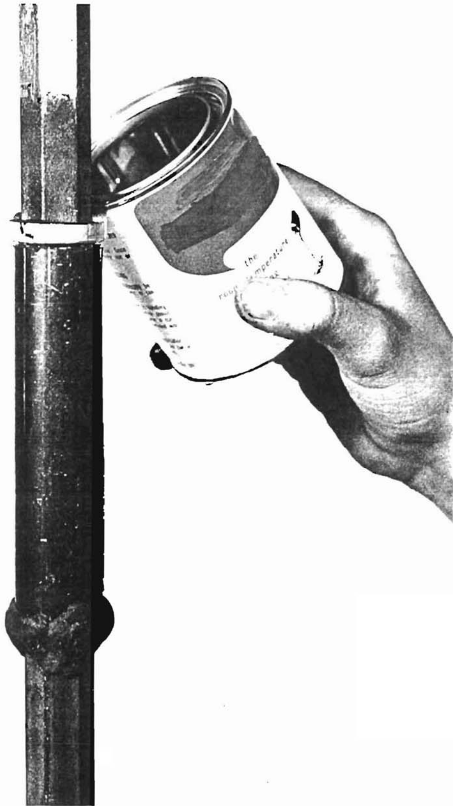
FIGURE B-21. - Filling a tube with liquid Flexane.
