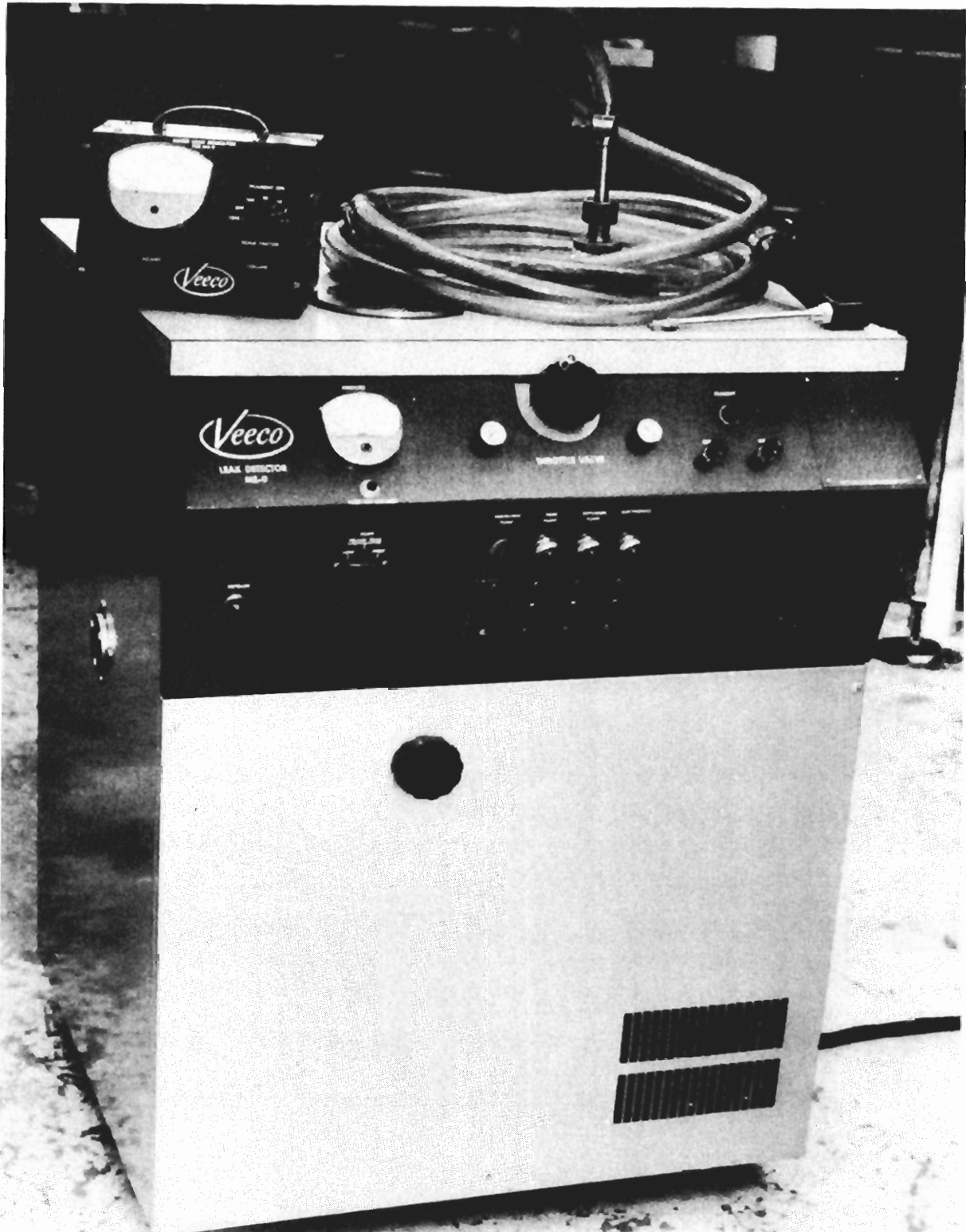
FIGURE 20. - Veeco MS-9A Helium-Leak Detector.
