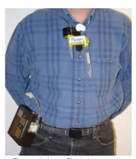
The sampler in use: The worker wears the sampler clipped to his shirt. The inlet of the sampler is close to the nose and mouth of the worker to ensure that the aerosol sampler is collecting the aerosol particles that the worker is actually breathing.
