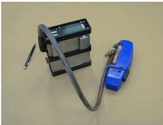
Figure 5. PDM-2 showing lapel and belt pack modules
