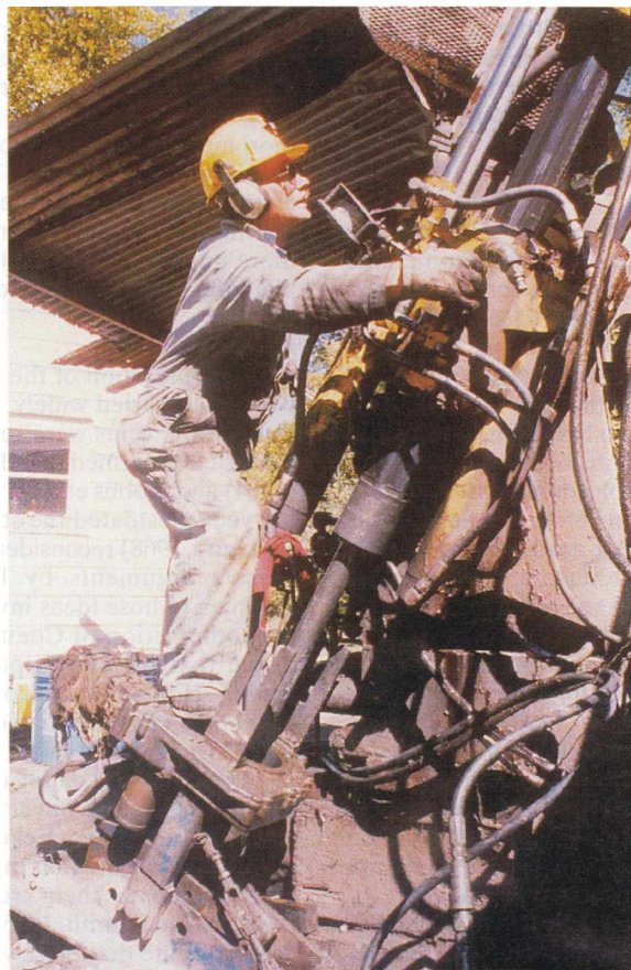
The Longyear 44 is commonly used for surface exploration diamond drill holes. Photo: Lisa Hardy, Sunshine Mining Co.
