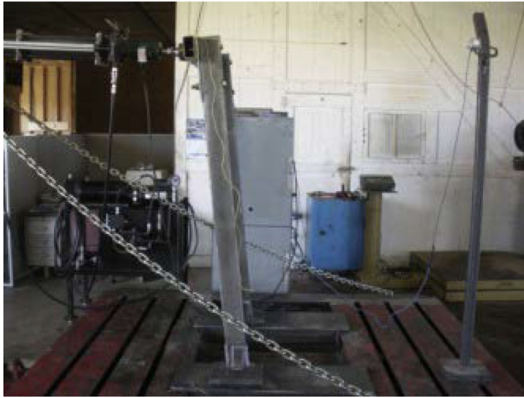
Fig. 2. Rear load test Long 460 ROPS.
