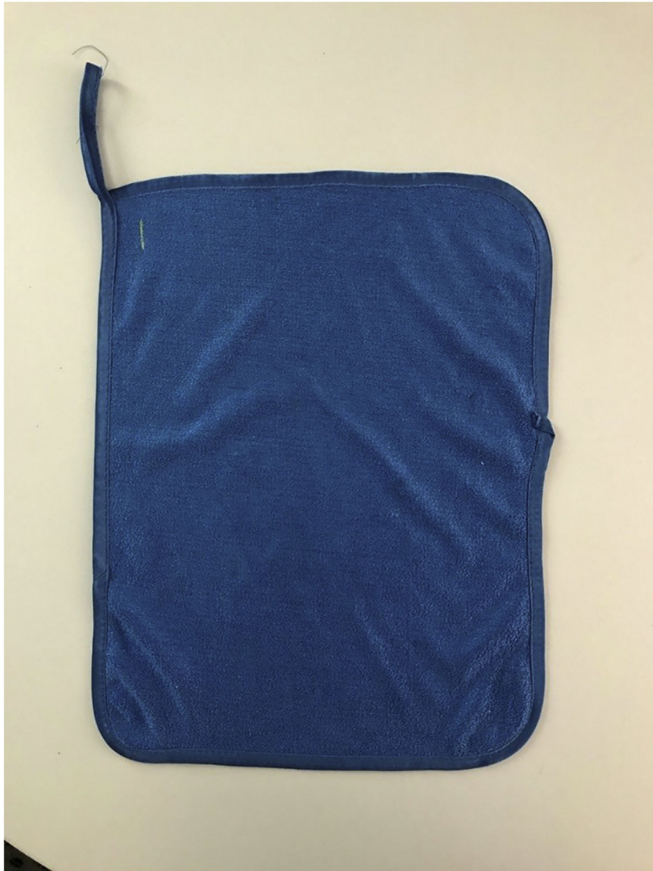
Fig. 1. Antimicrobial (treated) hand towel, 30 cm × 40 cm, with border consisting of untreated binding (untreated towel appeared identical).
