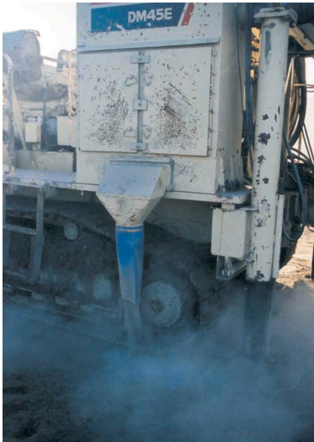
Dust (including the respirable size fraction) becomes entrained in the atmosphere from the dumping of fine material from the drill dust collector.
